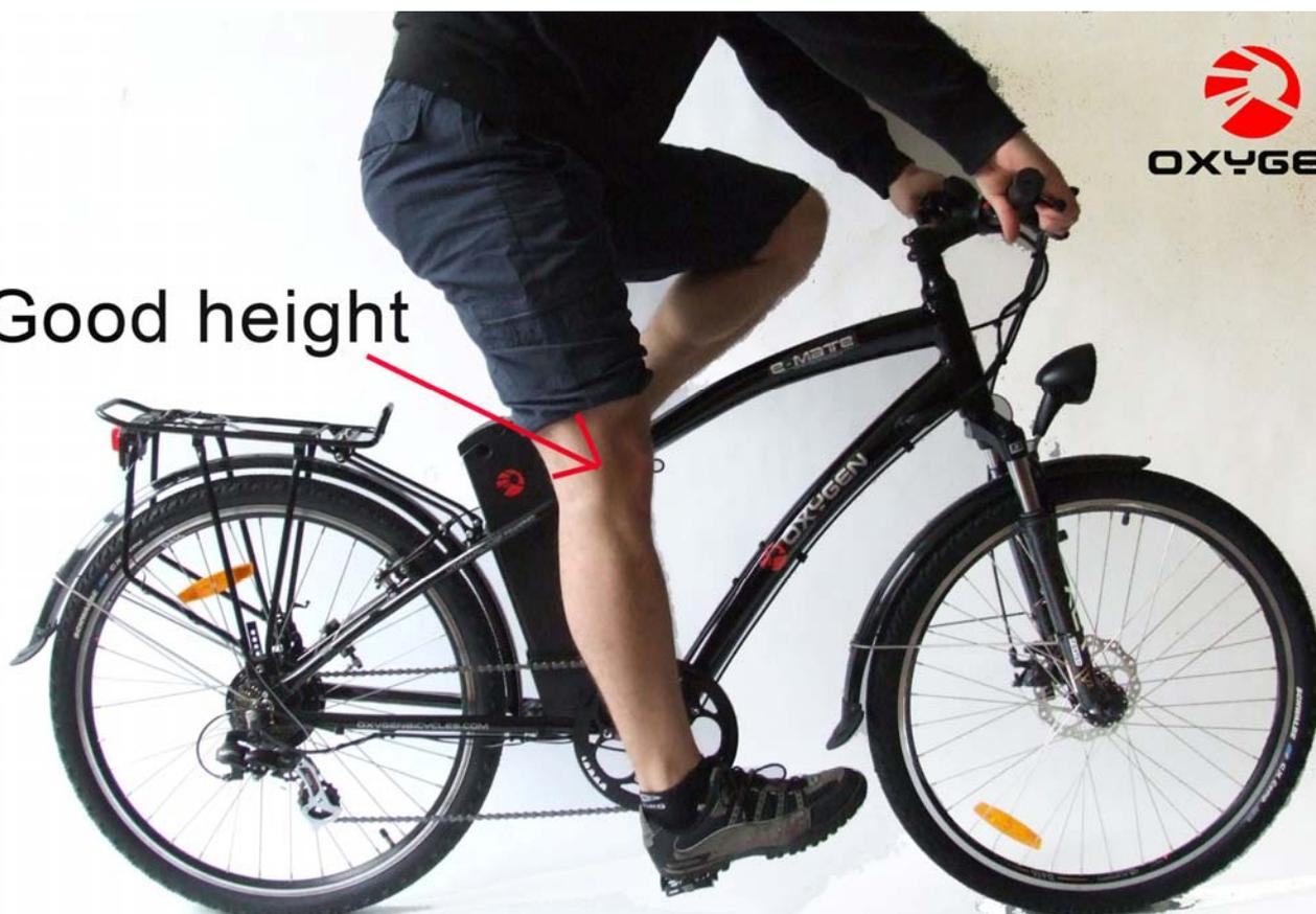
While adjusting the seat height please note that each seat post has the safety marking on the seat pillar. Please do not exceed the border of safety in any circumstances. The markings on the seat pillar always need to be hidden in the seat tube and never exposed above it. Seat post adjusted above its acceptable limits may cause the personal injury as well as the damage to the frame.
